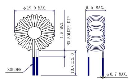
\* Dimension does not include solder used on coil.
